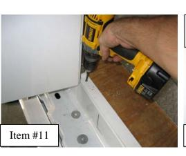
Attach the doorframe to the vehicle using #10 x 1" Phillips pan head sheet metal screws
